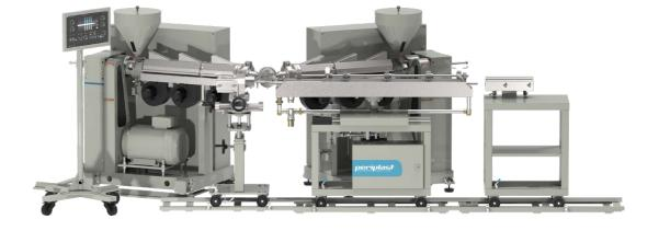
Periplast Spiral Medical Tube line for the production of spiral breathing tubes. These tubes are made of PVC-soft for the hoses on which a PVC-hard spiral is applied during the production. The extruders are particularly used for the manufacturing of medical catheters with a diameter of 15 to 19mm. The line consists of 2 extruders (PVC-soft and PVC-hard), co-extrusion dies, calibrator, dual cooling (with adjustable inflow channel), automatic cutter and hose store.
