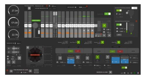
The main page designed specifically for each line including all the machines, sensors, and controls.
