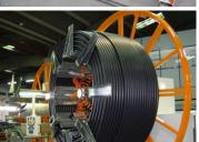
Linear speed "automatically synchronized" with extrusion speed controlling pipe tension
