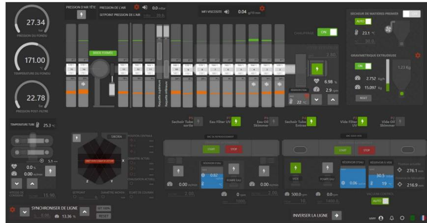
The main page designed specifically for each line including all the machines, sensors, and controls.
